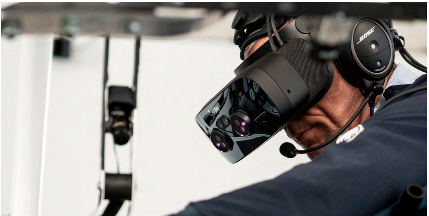
VARJO VR Head Mounted Display (HMD) and BOSE A20 Headset (Picture: VRM Switzerland)
