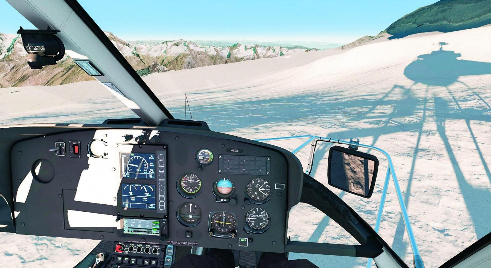
**Mountain landing site “Alphubel”:** The simulator’s visual system provides 3D vision with unprecedented resolution and imaging of the special lighting conditions.
